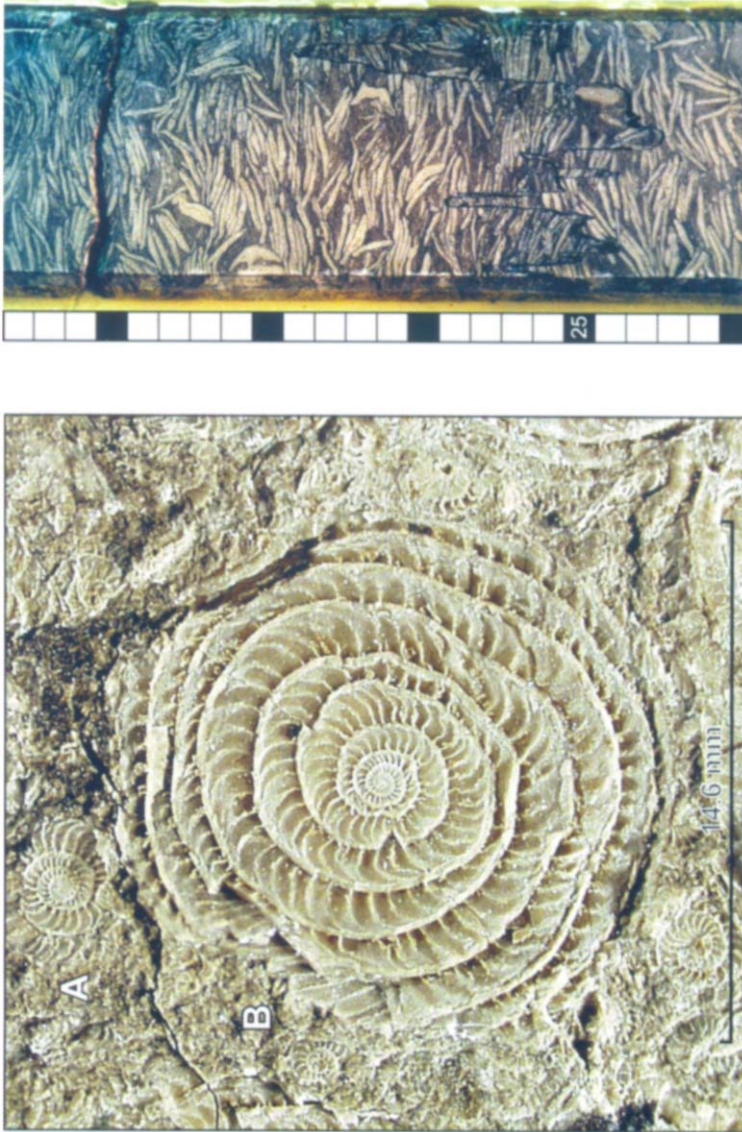
Core Slab from offshore Tunisie Hasdrubal Field, showing oil-stained stylolite. B-Form Nummulite rich El Garia Formation
