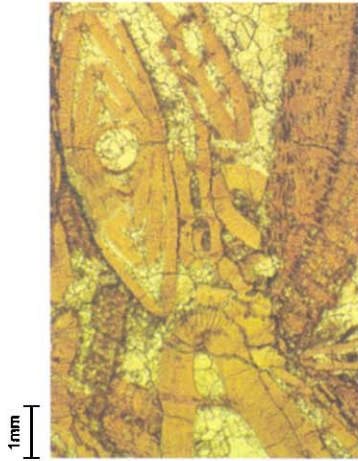
Hasdrubal-3. Nummulitic limestone with large Discoeyclina (bottom) and A-form nummulite (top right). Porosity is occluded by late calcite cement whilst compaction related fractures and associated pressure solution at grain boundaries is clearly visible.
