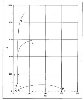
Fig. 6. Van Krevelen diagram for the Isle of Man samples.
