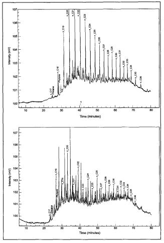
Fig. 7. Gas chromatogrammes (a) of sample *IOM 3* from the *Shellag Point* borehole; and (b) sample *IOM 5* from the *Ballavaarkish* borehole.
